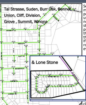
Sewer lines will be cleaned during the month of May. A cleaning nozzle is propelled from one manhole to the next using water under high pressure. The nozzle is then pulled back to the starting manhole. As the nozzle is pulled back, water scours the inside of the sanitary sewer pipe. Any debris in the pipe is pulled back with the water. If roots are found, they are cut with a root cutter. This process is repeated on every sewer line cleaned.
