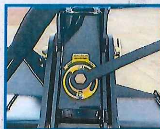
MDS furnishes a custom made wrench used to adjust the Acme Threaded Jack Screw.
