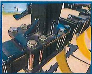
Sixteen (16) Grade 8 Bolts are used to keep the cross tube from sliding side to side.
