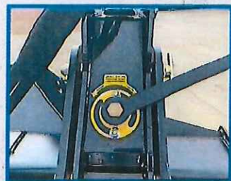
MDS furnishes a custom made wrench used to adjust the Acme Threaded Jack Screw.
