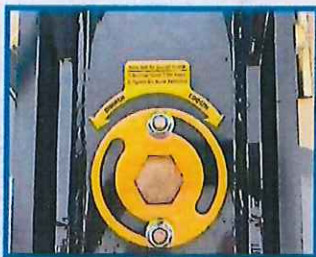
The patented Acme Threaded Jack Screw is used to adjust the retaining pin for easy removal.
