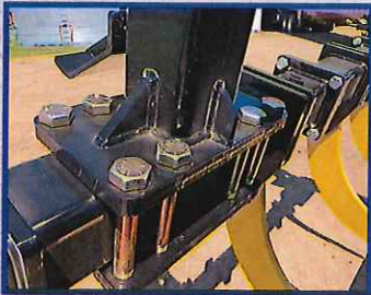
Sixteen (16) Grade 8 Bolts are used to keep the cross tube from sliding side to side.
